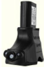
The Taser Cam is used with the Taser X26 model. It integrates into a rechargeable X26 power supply that is inserted into the handle, and records audio and video once the device's safety is moved into the off position. The information is then downloaded with a USB cable. The device allows for documentation of the incident as well as accountability (Taser Products).
