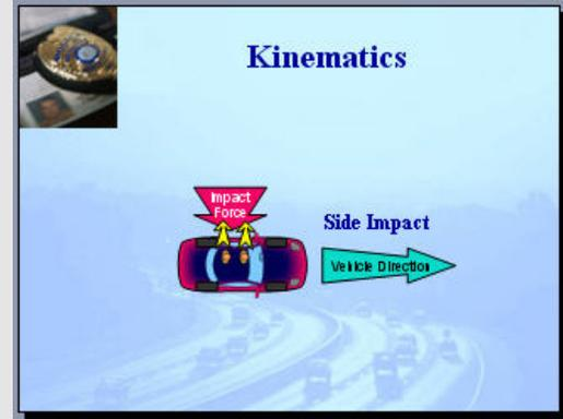
**Instructor Note:** Lateral impact can result in substantial penetration of the passenger compartment, and can represent a greater danger due to lack of space available for crush offered by frontal or rear-end crashes.
