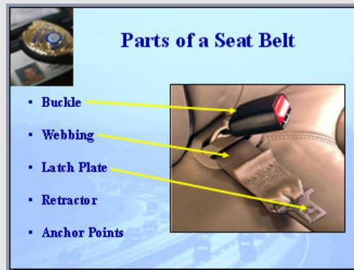
**Webbing:** The fabric of the belt, which secures the occupant to the vehicle during a crash and extends the time that the deceleration forces are experienced by the occupant, allowing the occupant to “ride down” the crash.
