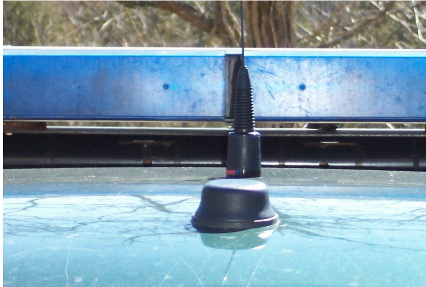
Picture 2.1 GPS Roof Receiver
