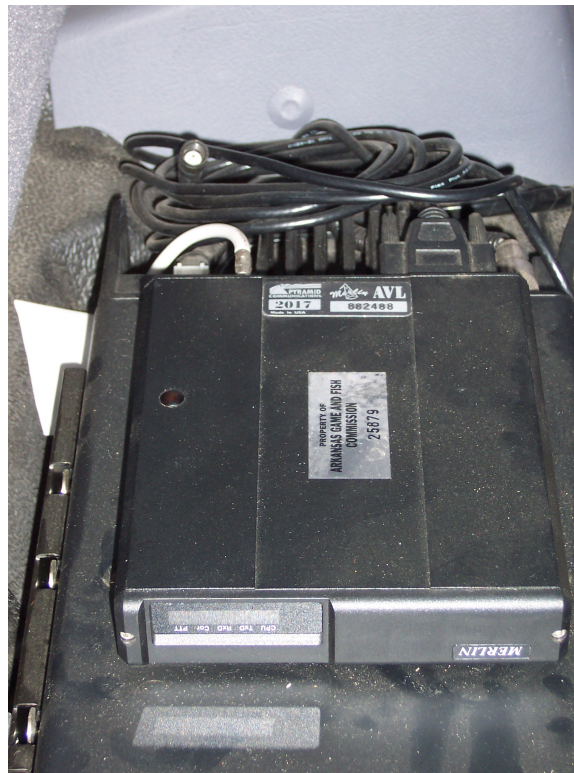
Picture 2.2 Merlin AVL system on AGF patrol vehicle
